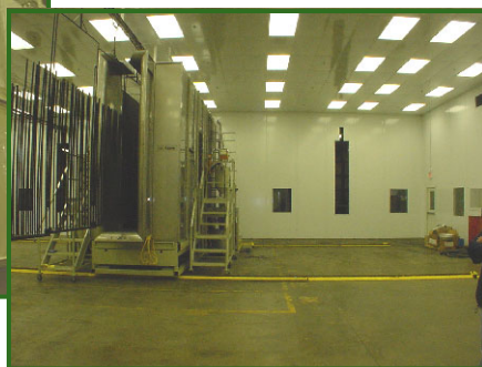
Movable powder spray booth to accommodate three paint lines.
