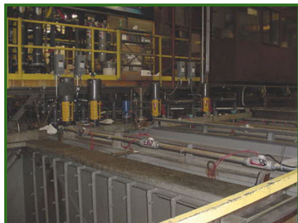
The modified e-coat line at Kohler's manufacturing facility for generator and electrical control parts.
