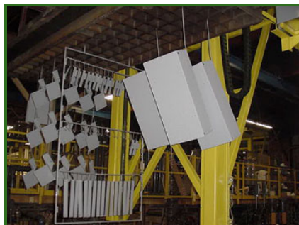
The modified e-coat line at Kohler's manufacturing facility for generator and electrical control parts.
